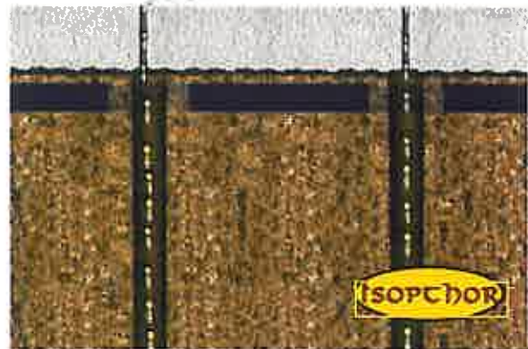
Termites Taking Advantage of Gaps In a Barrier
